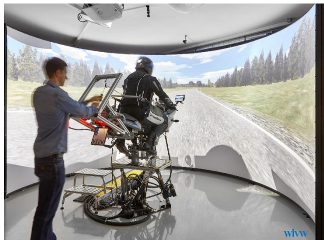
Advanced dynamic motorcycle riding simulator DESMORI at WIVW is being set up by project leader Sebastian Will
