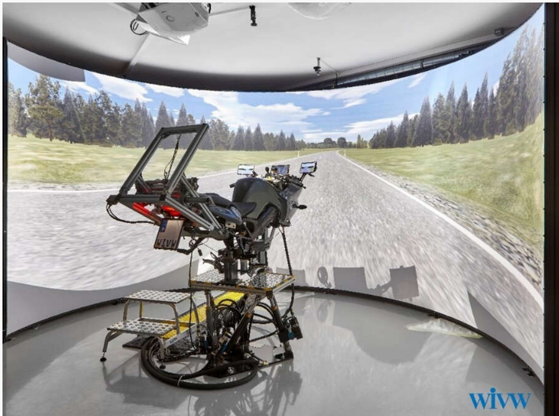
The dynamic motorcycle riding simulator at WIVW that was used for the study
