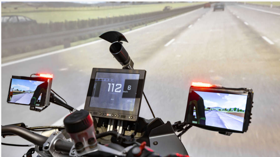
Red flashing LEDs mounted on the mirrors were used as Imminent Crash Warning
