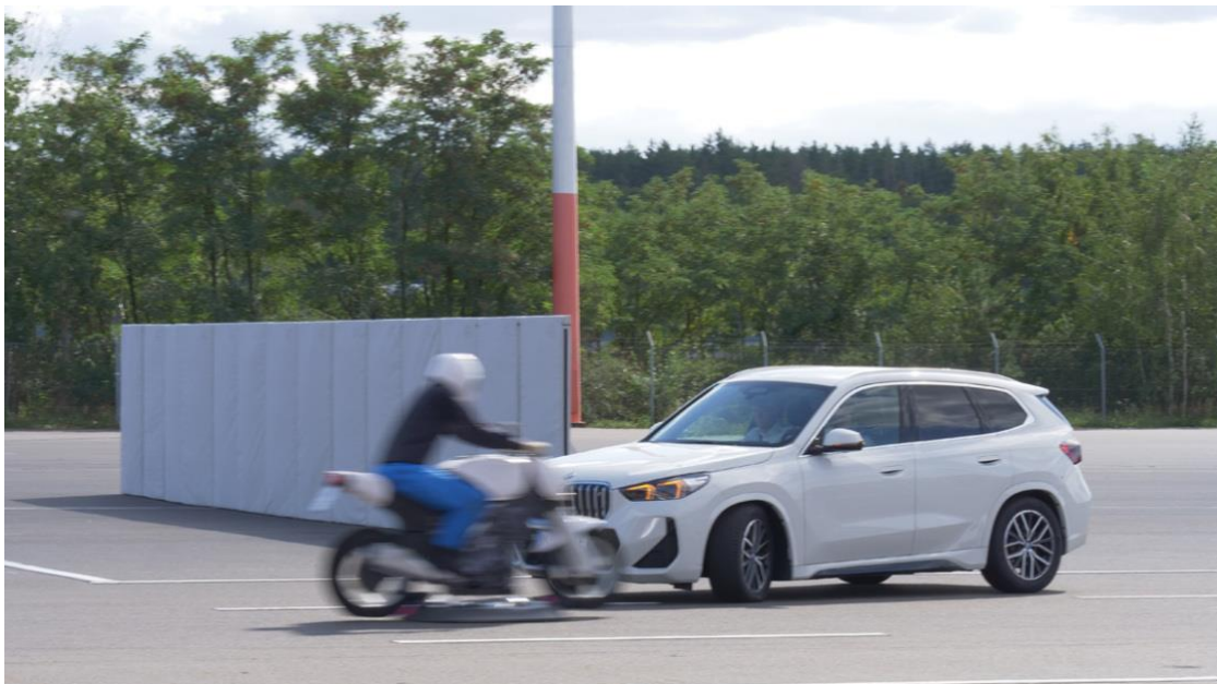
Systems working together to support automated emergency braking: A forced braking by ADAS avoids a collision with an oncoming motorcycle
