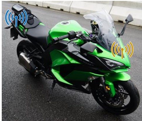
Figure 13: Mounting positions of the antennas
