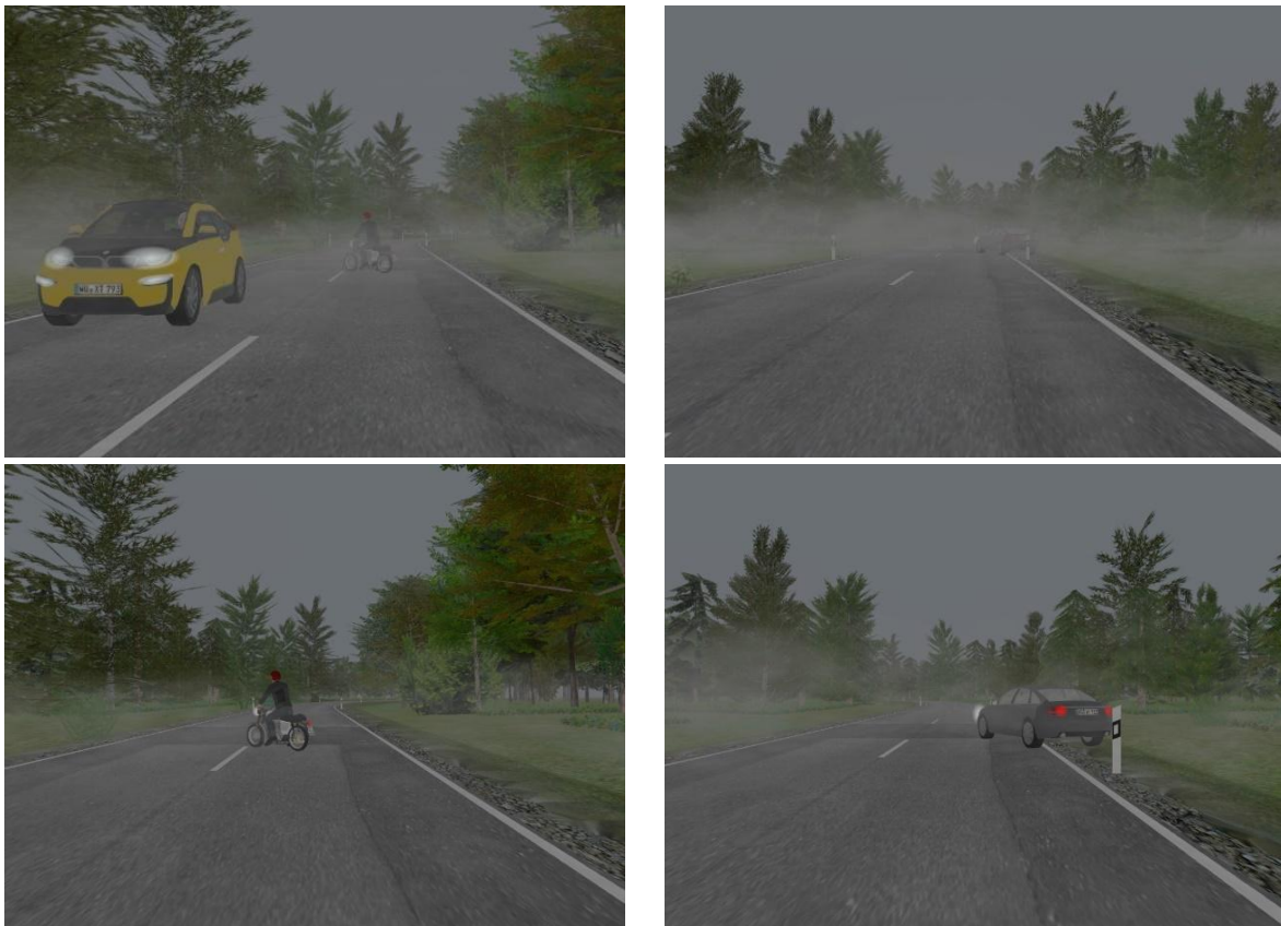
Figure 2: Local Hazard Warnings: PTW (left) and passenger car (right) test scenario with obscured obstacles due to ground fog (upper row) and recognisable obstacles when approaching the test scenarios (lower row).
