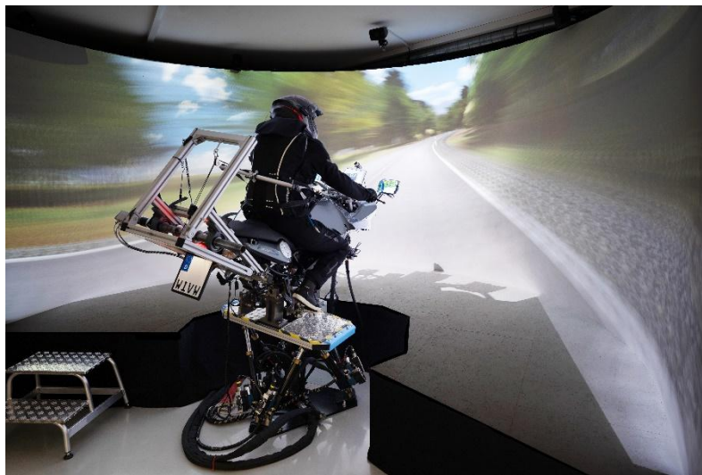
Figure 1: DESMORI dynamic motorcycle riding simulator at WIVW.
